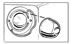
The oven lamp(bulb) is covered with a glass removable cover which is held in place with a bail-shaped wire.
